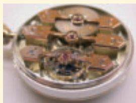
GP Tourbillon under three bridges Ø30 mm – Restoration
